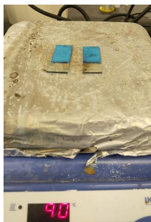
Fig. 3: Annealing process of the coated FTO glass at 90^\circ\text{C} .
